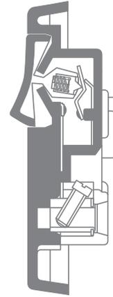
Unique labyrinth switch design minimises visible arc flash and prevents front access to live parts.
